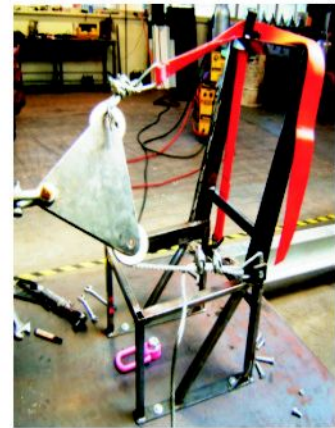
TSV developed test rig for full load testing of seat frames and anchorages.
